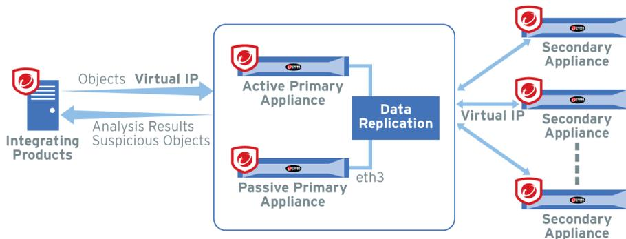
**FIGURE 2-3. High Availability Cluster with Load Balancing**
