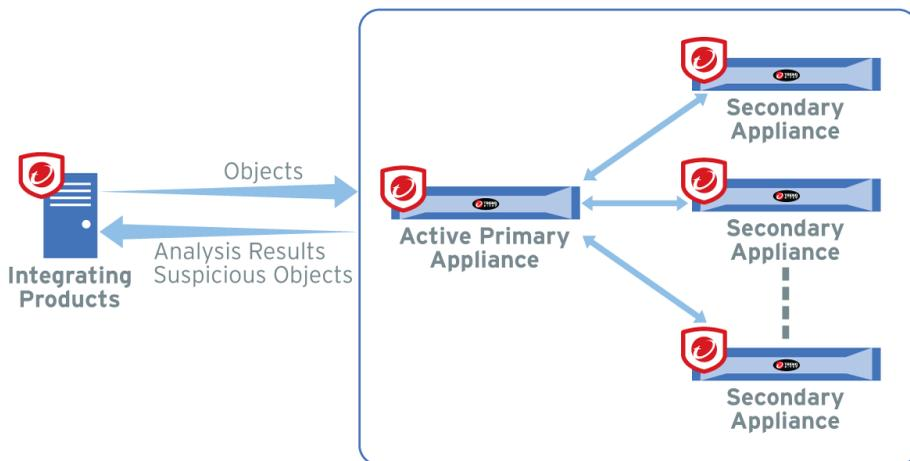
**FIGURE 2-2. Load-Balancing Cluster**
