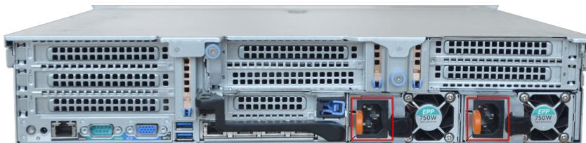
**FIGURE 3-2. 1200 appliance AC power slots**
