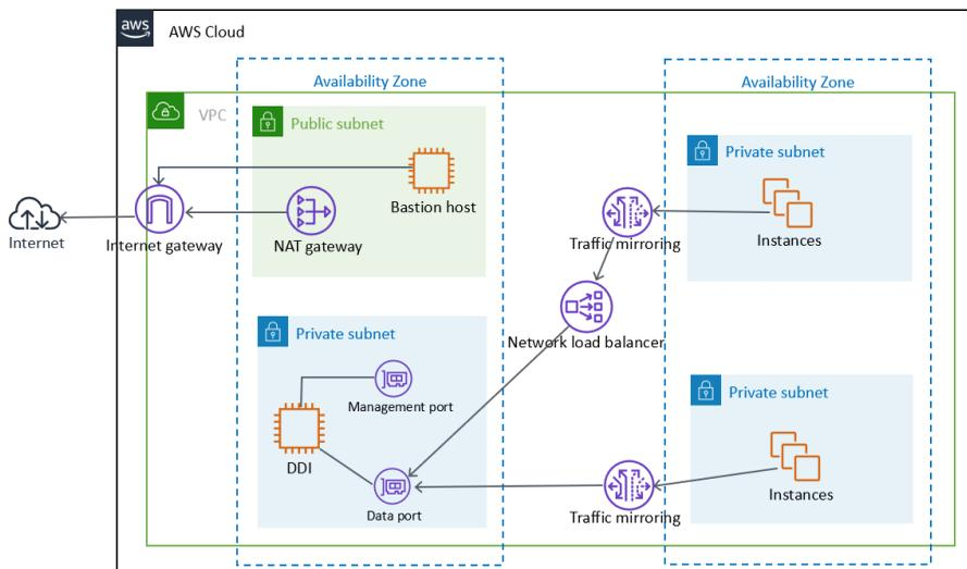
**FIGURE 2-1. Deployment Architecture**
