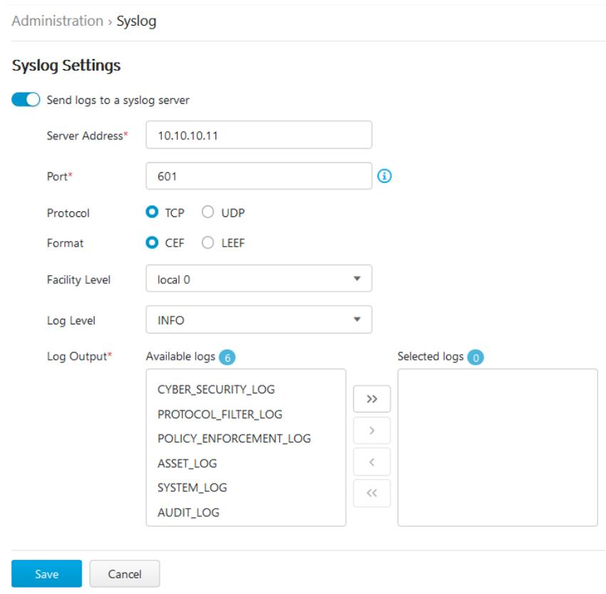
The screenshot shows the 'Administration > Syslog' configuration page. The 'Syslog Settings' section is active, with a toggle for 'Send logs to a syslog server' turned on. The configuration fields are as follows:
