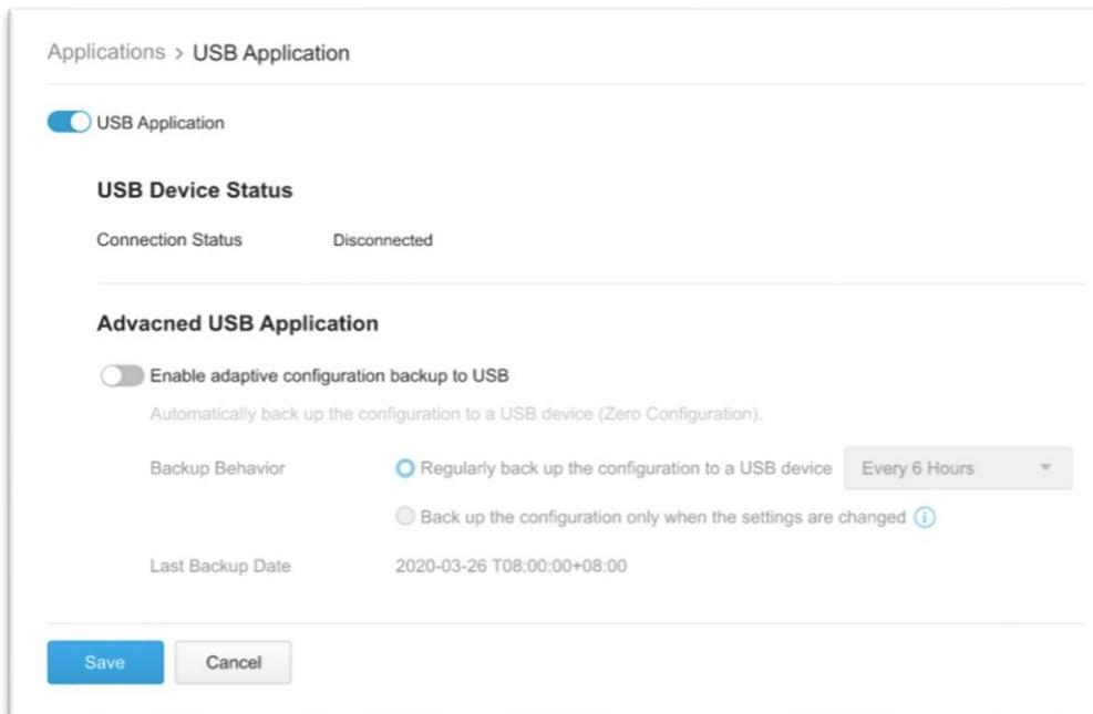
3. Use the toggle to enable USB Application usage by enabling the USB port.
