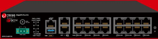
EdgeIPS Pro 216 is a Transparent Security Appliance, supporting up to 8 pairs of IPS segments. Users can efficiently adapt the rack mounted EdgeIPS Pro 216 into a flexible solution for the challenges of Ethernet communications.
